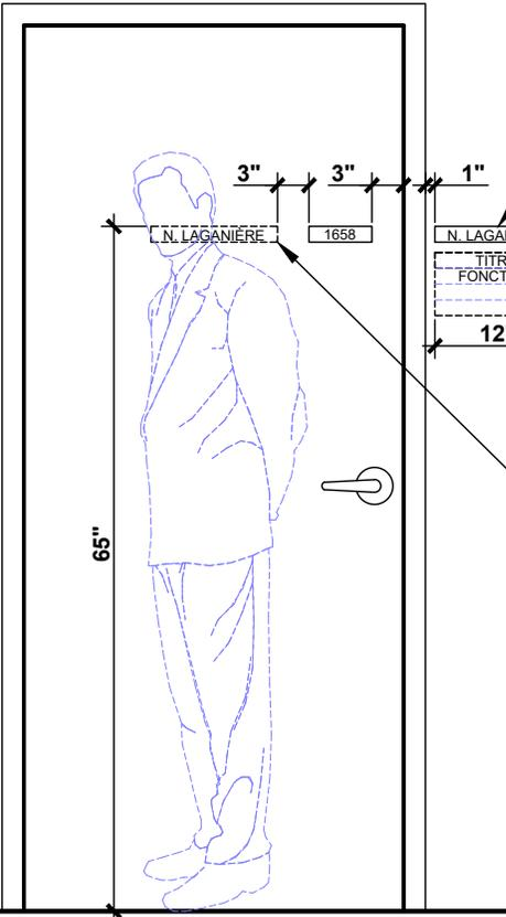
DANS UNE SITUATION OÙ LA PORTE EST EN RETRAIT DANS UN ESPACE LIMITÉ (ALCÔVE) PAR RAPPORT AU MUR, LA PLAQUETTE D'IDENTIFICATION DOIT ÊTRE INSTALLÉ SUR LE MUR SELON INDICATION.
