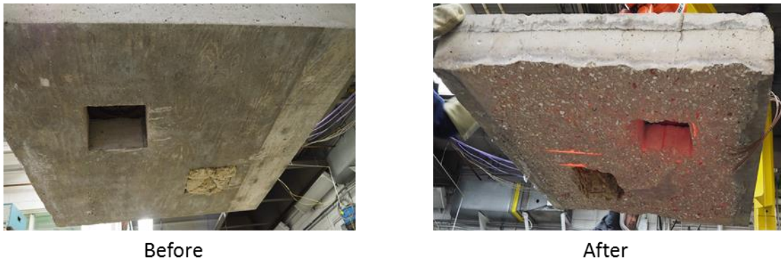
Figure 11. Photos of the exposed surface of the slab before and after the test.
